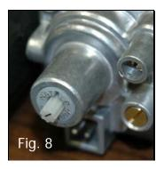
The step motor modulates the flame height at six (6) different levels and automatically calibrates itself to zero when power is first applied via the wiring harness.
