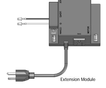
The "Main Control Module" acts like an "Operating System" of a computer and controls all primary functions of the IPI system (i.e. Extension Module and IPI Gas Valve). The "Extension Module" controls the fan and auxiliary lighting powered by 120VAC. The IPI gas valve lights the intermittent pilot and burners of the fireplace. While the hand held transmitter is programmed to remotely operate the main control module.
