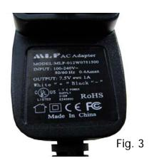
AC adaptor is a transformer that converts VAC to VDC power. Ensure the electrical circuit you are using has 120VAC power. The adaptor is rated at 7.5 VDC and must produce a minimum of 5.4 VDC in order to operate an IPI system.
