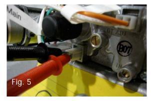
6. Check the resistance of Main burner coil at the gas valve. Remove the 2-pin connector labeled MAIN from the gas valve. Using a multi-meter touch one lead to each pin and measure coil resistance. A good reading should be 990-Ohms to 1230-Ohms. If the resistance falls outside of these limits, replace the gas valve. See fig. 6.
